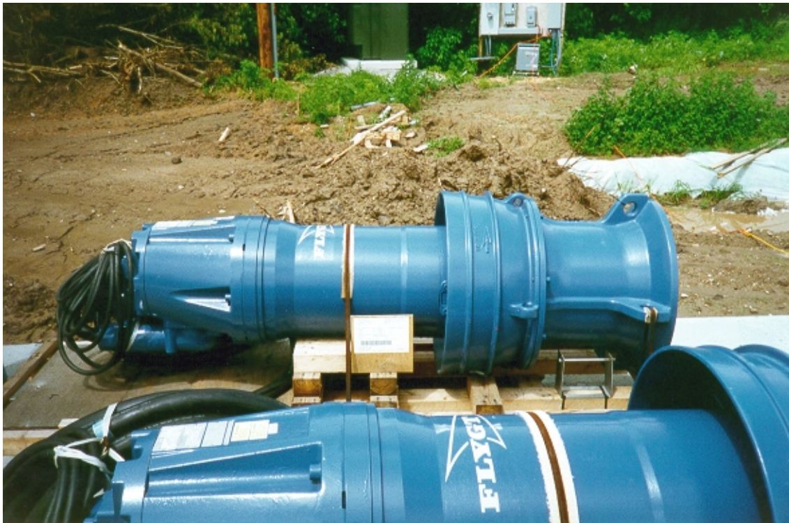
Figure 3-11. Large submersible pumps
